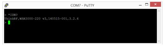
7. Refer to the WSA5000 Programmer's Guide that is associated with the firmware release of your WSA5000 for the SCPI commands to use with your WSA5000 via the USB console terminal window. The firmware release version of your
