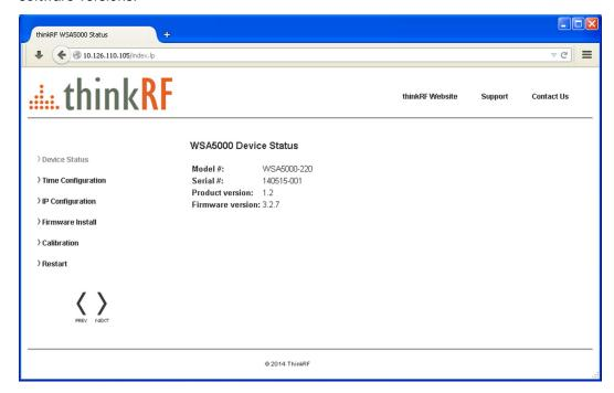
Note that if you have product version 1 with firmware image v3.2.6 or earlier, the "Product version" field would be labeled as "Hardware version". This field is important for selecting the correct firmware image to update, i.e. product version 1 can only be updated with firmware v3.2.7 or lower; and product version 2 with firmware v4.0.0 or higher.
