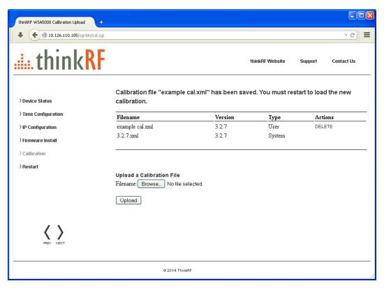
**5.** Restart the WSA5000 by using the administrative console or toggling the power switch. The boot up will take longer than usual after the restart as the embedded system applies the new calibrated values.
